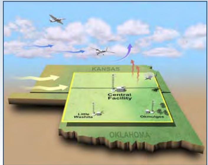
*During CLASIC, a fleet of seven research aircraft and enhanced surface instrumentation were used to obtain cloud and atmospheric properties measurements throughout the SGP site, which covers 55,000 square miles in Oklahoma and Kansas.*
